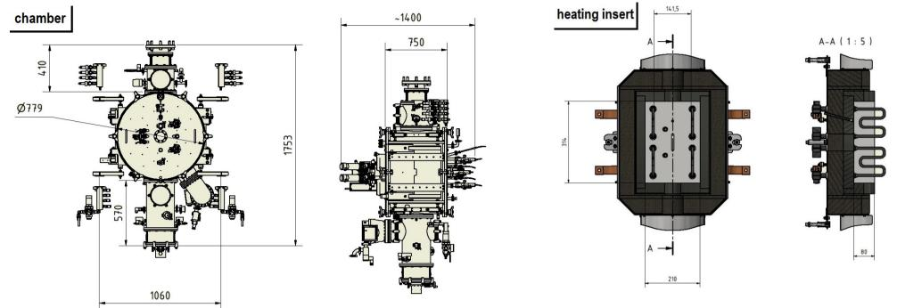
The chamber is designed as a horizontal cylinder. The complete system is double-walled and water-cooled. In order to compensate for heat-related dimensional changes, one half of the heating insert is spring-mounted
