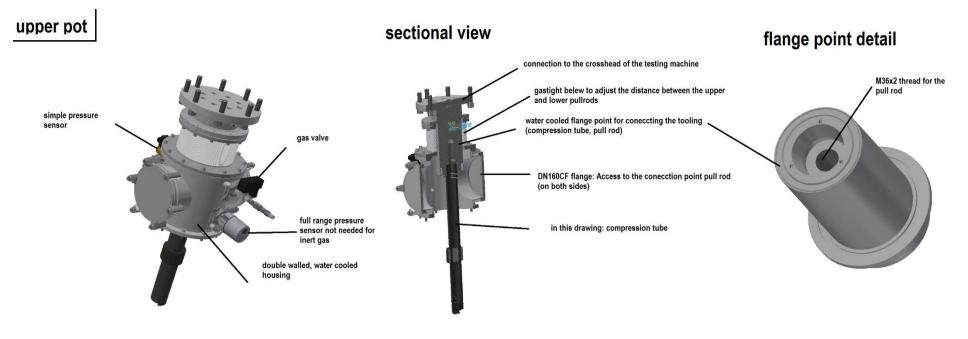
The DN160 CF flanges on both sides of the upper and lower pot allow the pull rods to be changed easily without having to "crawl into the machine".
